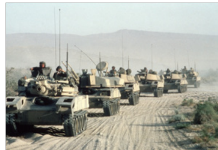
M551 Sheridan light tanks cross the desert during an Opposing Forces exercise at the National Training Center. The tanks have visual modifications designed to make them resemble Soviet armor, 1986. (U.S. Army photo)
